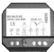
Receiver (48 x 51 x 28 mm) with ON/OFF radio frequency transmitter (controlled by radio-waves) with hidden installation. The receiver receives the radio orders emitted by the digital chronothermostat. It receives the orders and information wirelessly via radio waves. It can be associated to radiators and towel warmers.
