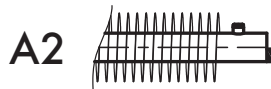
Atypical connection for FA1 and FAO radiators with a diameter of 57 and 76 mm.
